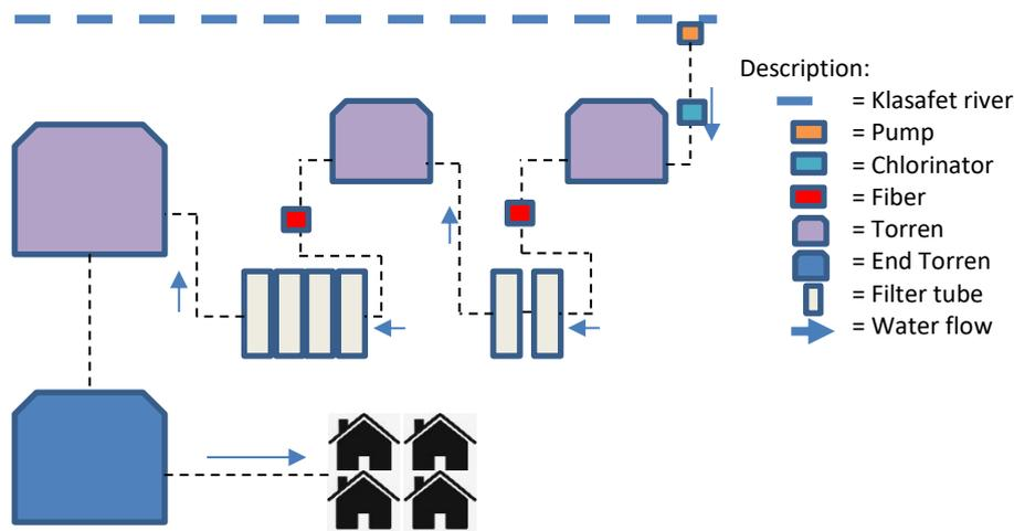
**Figure 1 Mechanism of Clean Water Flow**
